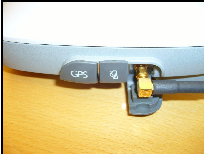
Figure 4. Connecting the SpaceCom IP221 Vehicle Antenna to the “active external antenna” connector on the Thuraya IP terminal.
